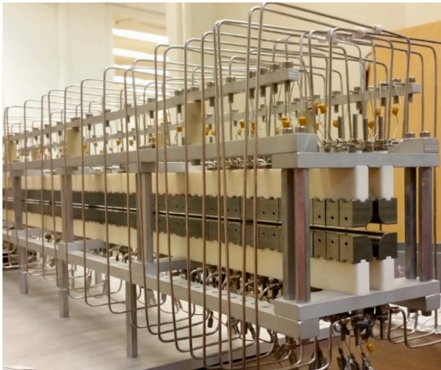
FIG. 4. A photo of the TAMUTRAP RFQ with in-vacuum electronics attached.
